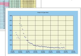
The ParticleTrak program logs the data directly into an Excel spreadsheet. Once the particle concentrations are recorded, the data can be organised, analysed, documented and printed for reports. The pre-programmed Excel graphs enable you to create descriptive reports for effective client presentations.
